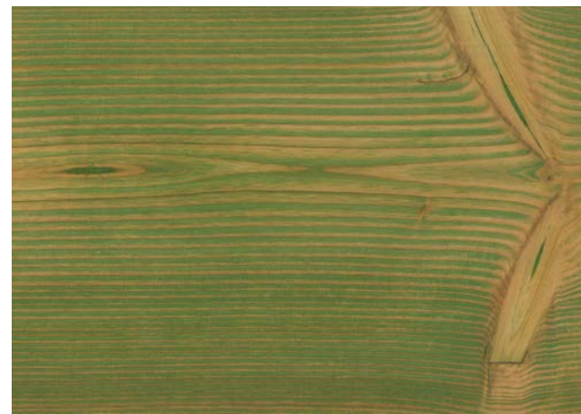
Sanded with 150 grain 1 × linseed oil, Chromoxid Green
