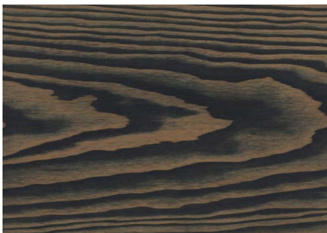
Sanded with 150 grain 1 × linseed oil, Dust Black
