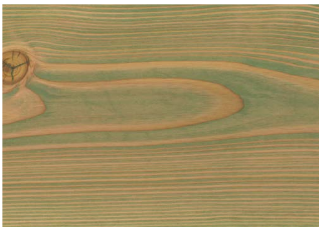
Sanded with 150 grain 1 × linseed oil, Verona Green
