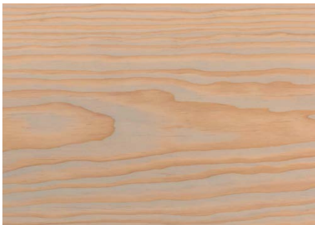
Sanded with 150 grain 1 × linseed oil, Light Grey
