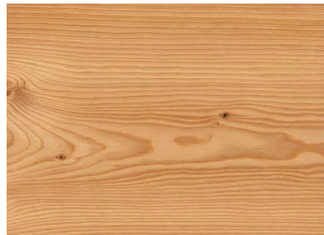
Sanded with 150 grain 1 × linseed oil, Nature
