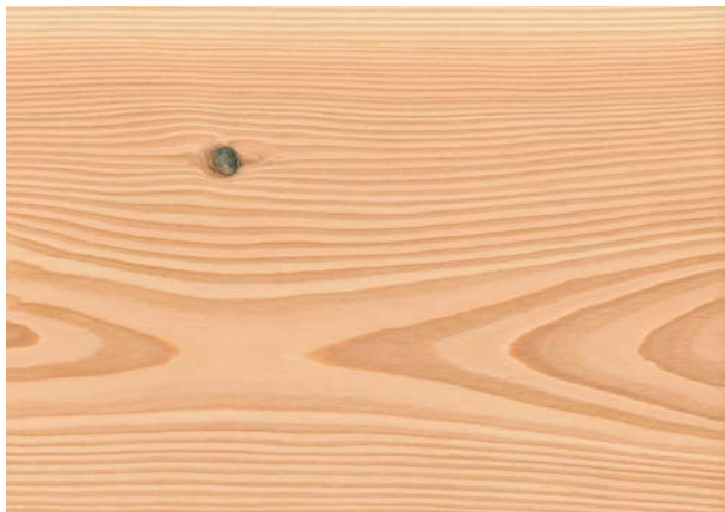
Sanded with 150 grain untreated
